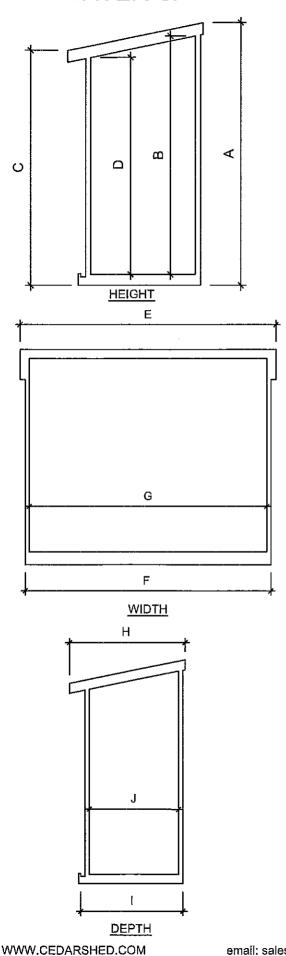
Western Red Cedar Shingle Roof All framing components are nominal 2"x3" in size 2"x3" floor joists on 16" centers Wood siding is Bevel Siding Window panel can be placed on front left or right side of the shed
